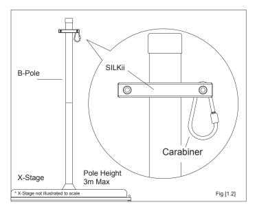
The SILKii should be installed at the top of the pole – over the X-Joint Hex Key hole as indicated - this could be done before the B-Pole is attached to the A-Pole, or a ladder will be needed. When installing on an X-STAGE, it is advisable to remove the B-Pole, then install the SILKii, before replacing the B-Pole. Additional weight is mandatory.
