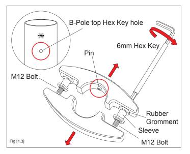
Remove the 2 x M12 bolts on either side of the SILKii – note the pin on one side of the SILKii. The pin locates into the X-Joint Hex Key hole at the top of the B-POLE. Undo each side evenly otherwise the SILKii will lock. Whilst loosening the screws, please ensure that they are not completely removed from the SILKii unit.
