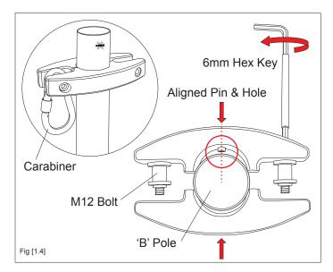
Attach the side with the pin to the pole. Once the pin has fully engaged with the hole. Line up the SILKii with the 2 x M12 bolts and fasten securely. Tighten screws progressively. If you over-tighten one screw, this will lock one side of the SILKii. Once correctly fastened, the SILKii is now in place and the Carabiner can now be attached.
