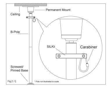
The SILKii can be installed at the top of an XPERT or SPORT pole that is mounted using a permanent fixing or on an X-Stage. SILKii MUST NOT be used on a stand-alone pole that is not secured using a permanent fixing/ceiling mount or a secured base.
